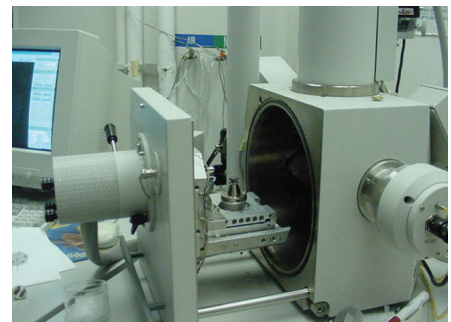
A modern SEM "electron microscope," showing the chamber open. The chamber will be sealed and the air removed.
